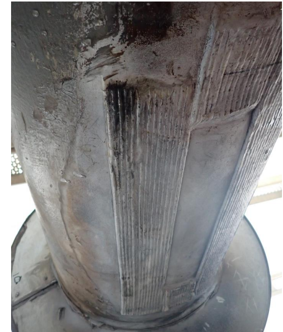
After Magnetic Particle Test – The entire welded area ground flat to ensure that Ultrasonic Examination could be performed
